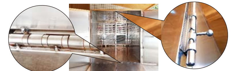
Use thick hinges and latches
