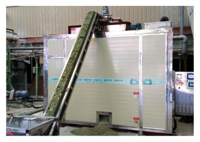
Sludge drying line (6-layers)
