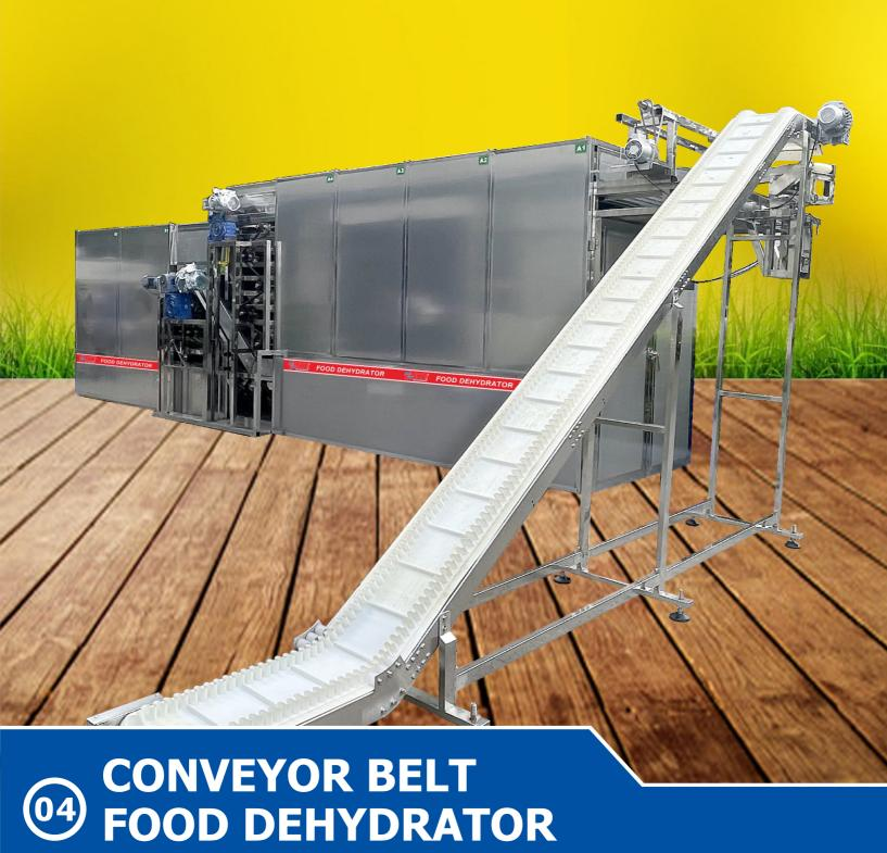
automatic continuous drying equipment for large-scale production
