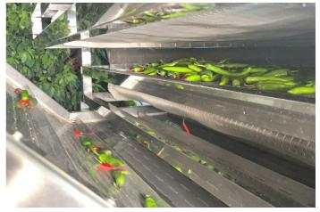
Flow lines can be used for large amount of material that can be dried in a relatively shot time. The running speed of the conveyer belt can be adjusted according to the food character.
