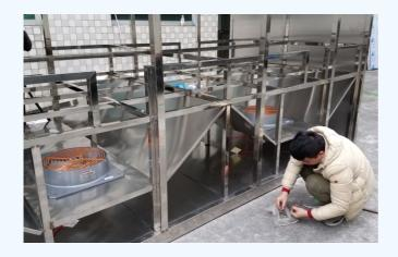
This specially structure good performance on drying the light product, such as the leaves, chives, some very easy to fly up in the drying process, we have made special mesh to cover the big tray and let them not fly and drying be better.
