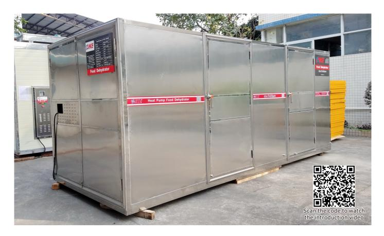
The AIO-500 series all-in-one dehydrating system used with IKE WRH-500 series drying machine. This type of dehydrating system is usually using specially big trays. For some round, no sticky items, we can dry them by direct stacking. The thickness of the material is about 300mm, the strong wind blows directly from the bottom and pass by the material.
